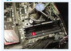
Turn off your PC and switch the power off at the wall but leave it plugged in. Earth yourself - for example, by touching a metal radiator. Open the case and lay it flat on the floor. Locate the memory sockets 11 and ensure you have clear access to them. You may need to move or unplug any cables that are in the way.
