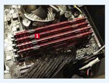
Add the rest of the RAM, 11 then put your PC back together again and power it up. The new memory should be listed on the boot-up screen. If it isn't showing the correct amount, follow the instructions in Step 1 to open your PC and make sure each module is seated correctly.
