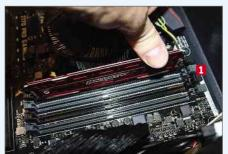
Open a memory slot by pressing down on the locking tab. If you're replacing existing RAM, pull out the module and set it aside. Insert your new memory module, making sure the notches align. It will only go in one way. Press down firmly until the locking tab 11 pops up, securing the module in place.
